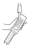
Make sure bin is completely dry. Reinsert filter and place bin back in the robot.
