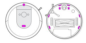
\* Important: Do not spray cleaning solution or water onto the sensors or sensor openings.
