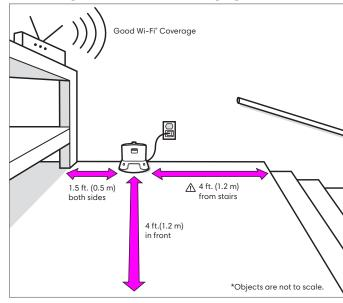
**MARNING:** To prevent the risk of your robot falling downstairs, ensure that the charging station is placed at least 4 feet (1.2 meters) away from stairs.
