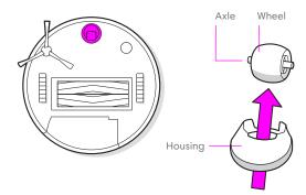
Important: A front wheel clogged with hair and debris could result in damage to your floor. If the wheel is not spinning freely after you have cleaned it, please contact Customer Care.
